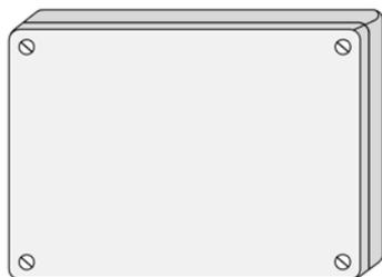
Intermediate terminal box for connecting a maximum of 4 air-handling units: (to be used outside the EX-range):
