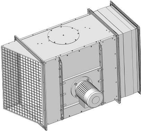
Horizontal motor shaft, with outlet protective grid PG BKF and flexible connection FLC BKF (WARNING: only allowed, if the motor is not exposed to elements. The motor has IP55, rain influence could be harmful. Snow freezing the motor cooling fan could cause starting problems).
