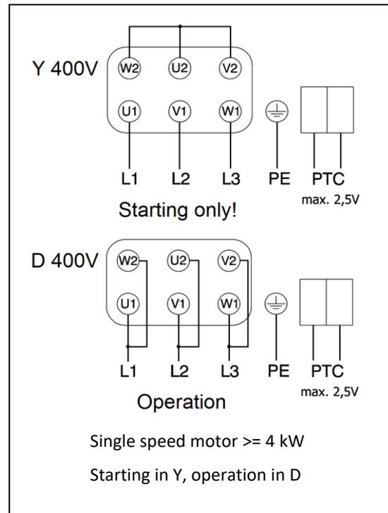
**\*Note 1:** two possible motor connections at 3 kW, 6 pole motor. Please observe the motor nameplate.
