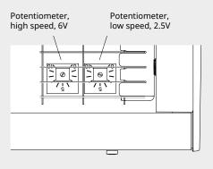
Internal potentiometer for low and high speed (accessible through the outlet grille).
