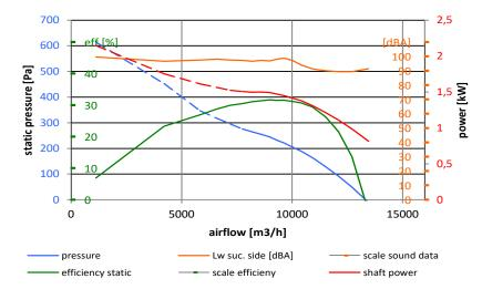
Measured in short casing with bellmouth without guard grille in installation type A according to ISO 5801.
